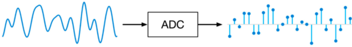
Figure 2: The digitization of an audio signal
